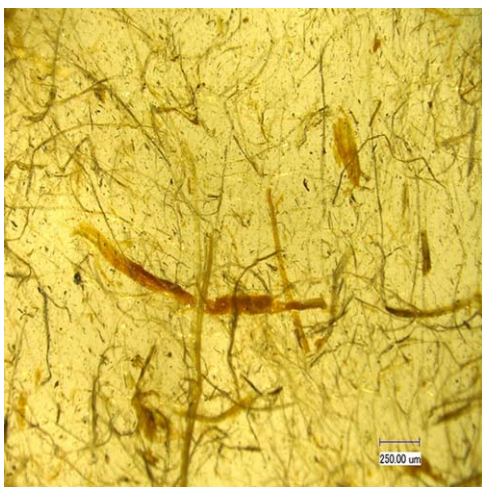
Figure 19. Microscopic sample of extruder (A) at 200 rpm and 30% Wf. [Color figure can be viewed in the online issue, which is available at wileyonlinelibrary.com .]
